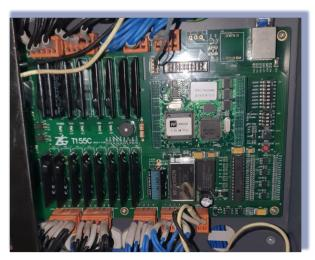
The T155 card replacement upgrade replaces all the functionality of the T155 cards and allows remote control of lateral and circumferential registration from a newly supplied console. The console includes a laydown area for the sheets as well a touchscreen and a keypad, either of which can be used to make register movements.
